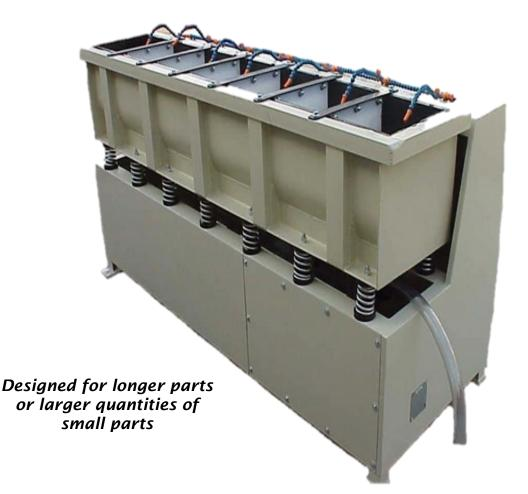
6 Cu. Ft. machine Tub: 76" x 12" x 14" Footprint: 60" x 35" x 36" 220 volt, 2 horse power, 3 phase motor\* Lining – hot poured urethane (industry standard) 5 gal. compound bucket, recirculation pump & pump hanger Holds 350 lbs. ceramic media or 200 lbs. plastic media (plus parts) \*magnetic starter not included
